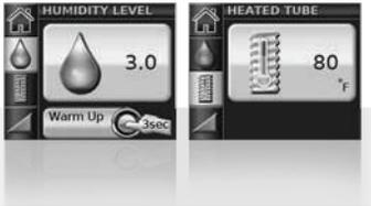
If enabled by the clinician, Climate Control can also be set to manual. In this mode, air temperature and humidity can be set independently, providing you greater flexibility but without the rainout protection guaranteed in Auto mode. In this mode, air temperature (61–86°F (16–30°C)) and humidity level (0–6) can be set independently. If rainout occurs, either increase air temperature or decrease the humidity setting.
