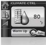
The recommended (default) setting for Climate Control is Auto mode. In Auto mode, you have the ability to adjust air temperature (61-86°F (16-30°C)) depending on preference. Based on your selected air temperature, Climate Control automatically adjusts the humidifier output to maintain a constant, comfortable humidity level of 80% relative humidity while protecting against rainout. In Auto mode the default air temperature is set to 80°F (27°C).
